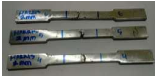
Gambar 6. Hasil pengujian tarik geser sambungan double butt lap joint variasi flux Harris (2 mm)
