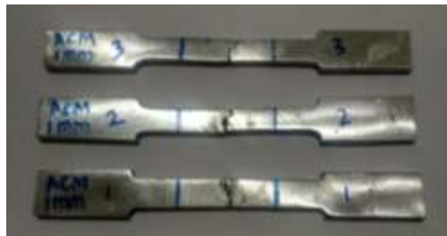
Gambar 4. Hasil pengujian tarik geser sambungan double butt lap joint variasi flux ACM (1 mm)
