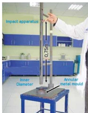
Gambar 8. alat uji determination of the adherence of the enamel to the substrate.
