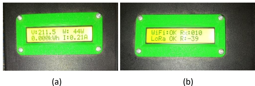
Gambar 9. Tampilan LCD sistem AMR: (a) LCD Node Sensor , (b) LCD gateway .
