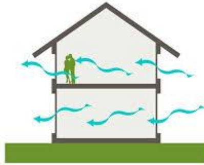
Gambar 43. Konsep Cross Ventilation
