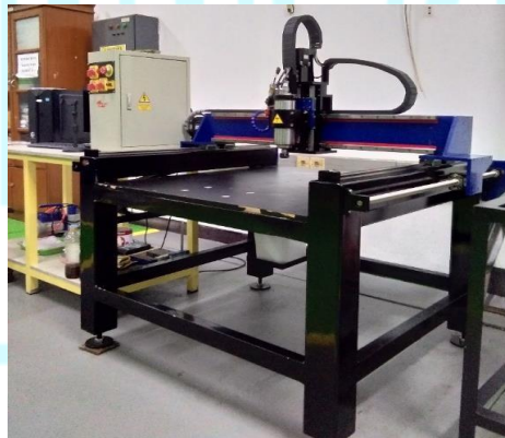
Gambar 2. Mesin CNC Milling Router 3 Axis
