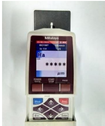
Gambar 3. Mitutoyo SJ – 210 Surface Roughness Tester
