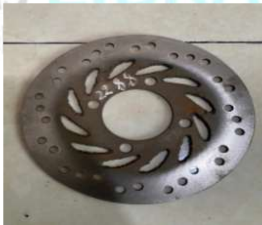
Gambar 6. Hasil machining rem cakram besi cor kelabu
