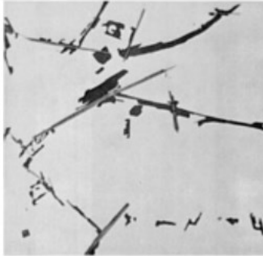
Gambar 11. Struktur Mikro Paduan Aluminium (ASM Handbook Vol.9,1992)
