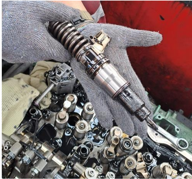
Gambar 3. 1.5 Proses Pengecekan Injector
