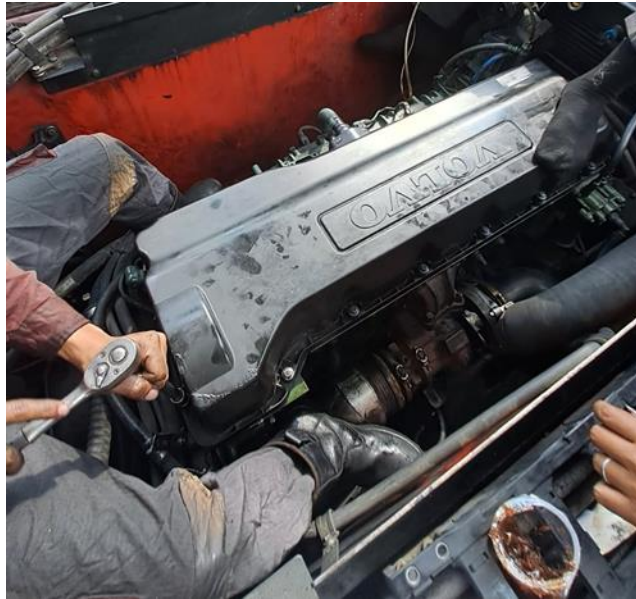
Gambar 3.1.14 Memasang Cover Engine
