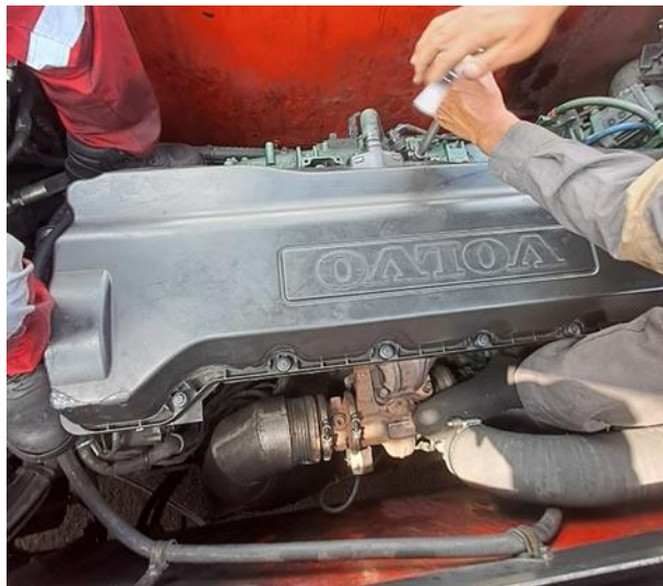
Gambar 3. 1.6 Membuka Cover Engine
