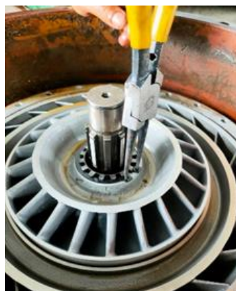
Gambar 6 Melepas Snap Ring Stator
