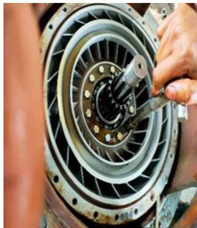
Gambar 7 Melepas Bolt Pump Impeller
