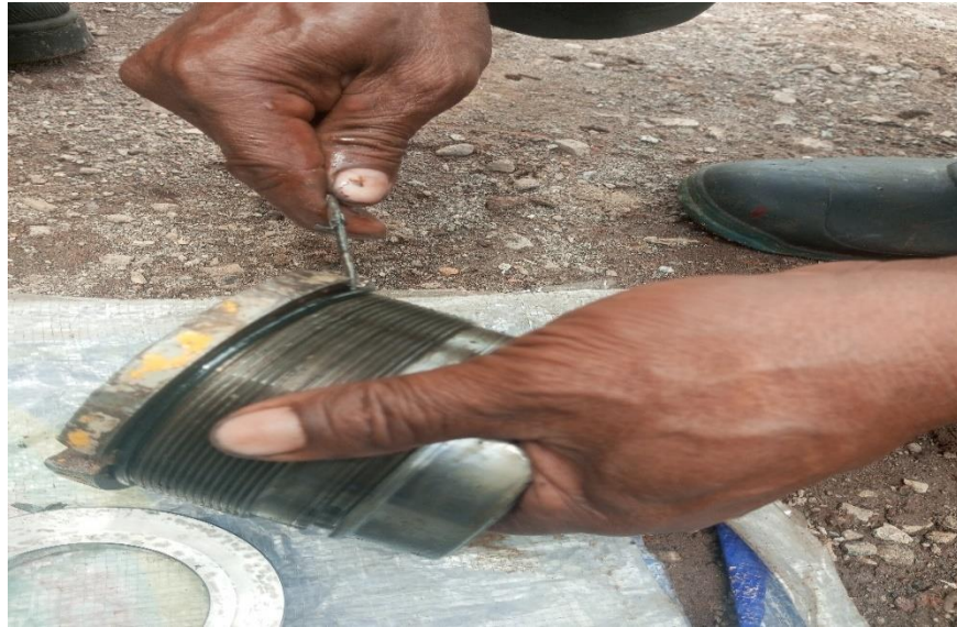
Gambar 4 Proses Memasang O-ring & Seal Cylinder Head (Sumber : Workshop Daya Kharisma)
