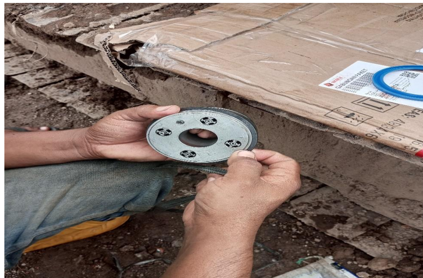
Gambar 5 Proses Memasang O-ring & Seal Piston (Sumber : Workshop Daya Kharisma)
