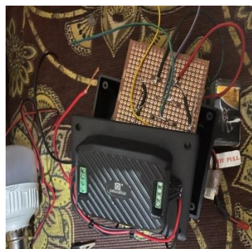
Gambar 8 Sensor PZEM Dc current
