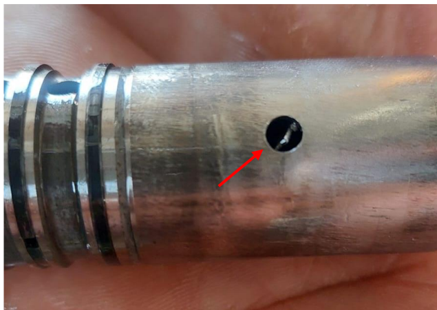
Gambar 4. Pengecekan Adjuster Main Pump
