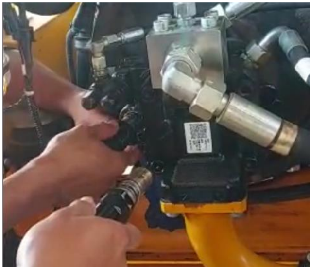
Gambar 7. Proses Pergantian Adjuster Main Pump Baru Serta Assembly
