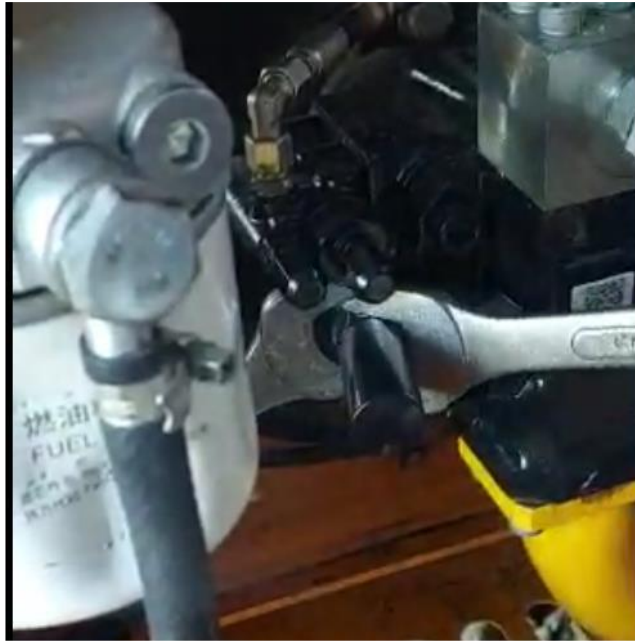
Gambar 3. Proses Melepas Adjuster Main Pump
