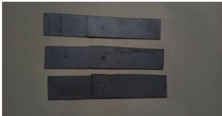
Gambar 3 Hasil Pengelasan Spot welding.
