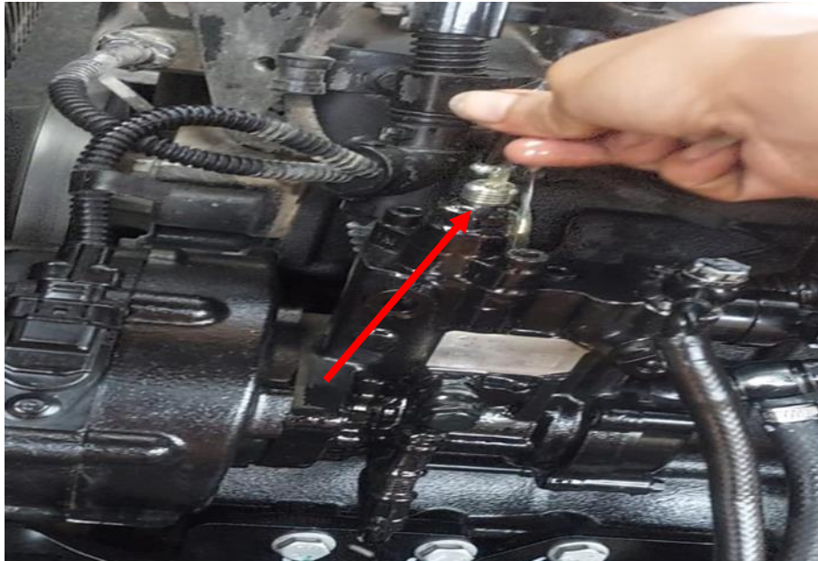
Gambar 2 Pengecekan Pressure Fuel pada High Pressure Pump
