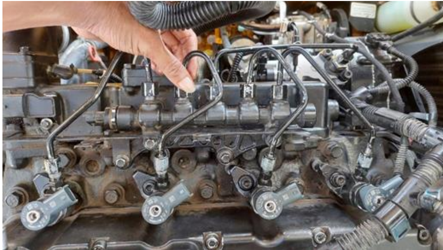
Gambar 6 Assembly pipa common rail
