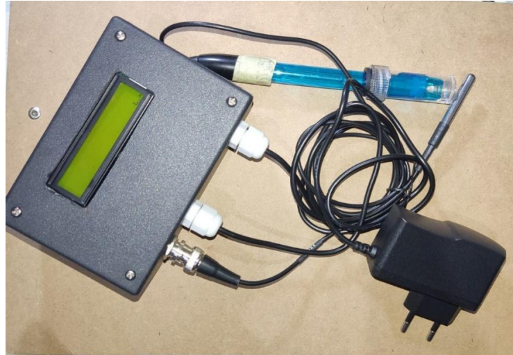
Gambar 5. Hardware sistem monitoring kualitas air kolam lele
