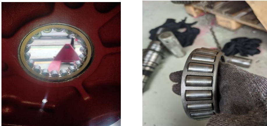
Gambar 4.17 Pengecekan visual terhadap bearing
