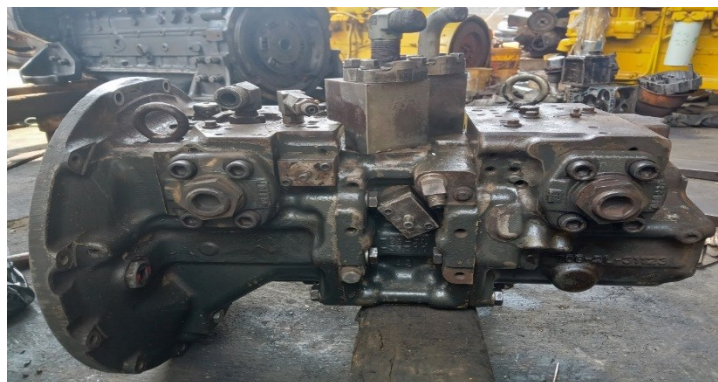
Gambar 3. Pompa Hydarulic Excavator Komatsu PC200-8
