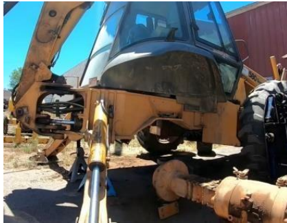
Gambar 14 Pemasangan Rear Axle
