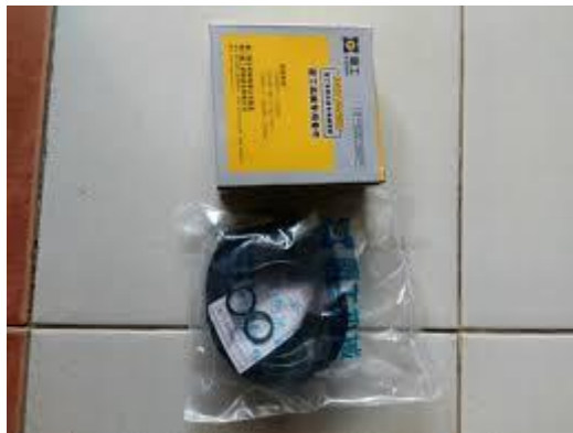
Gambar 11 Seal piston baru
