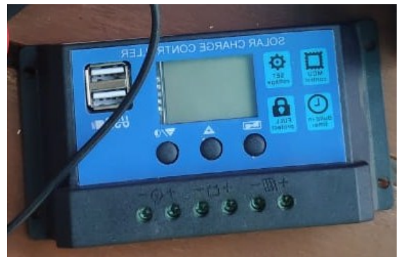
Gambar 6. Solar Charger controller
