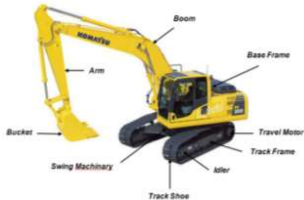
Gambar 3. Attachment Excavator dan Base Machine
