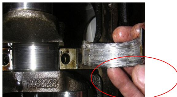
Gambar 8. Kondisi main bearing
