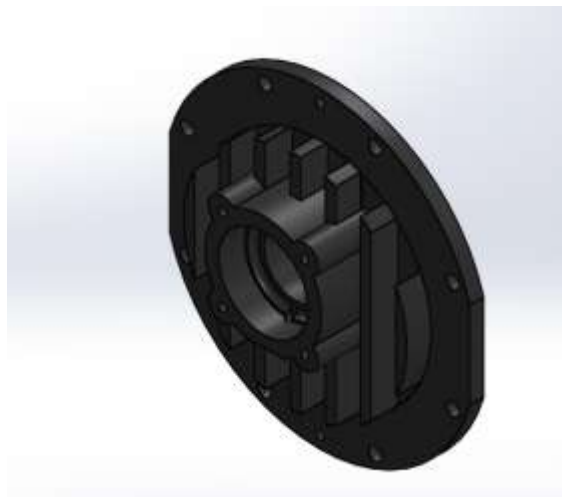
Gambar 7. Design 3D tutup pompa rotary sentrifugal CMM
