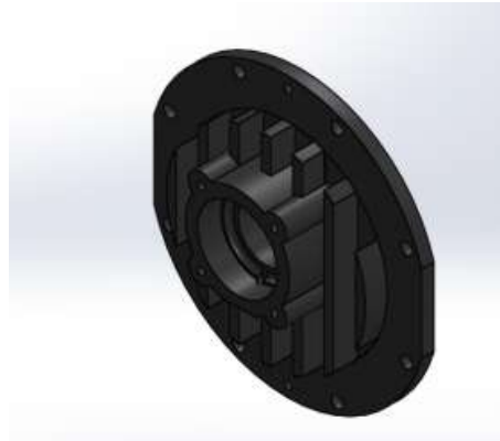
Gambar 4. Design 3D tutup pompa rotary sentrifugal manual
