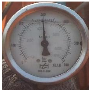
Gambar 2. Tekanan oil hydraulic 300 bar
