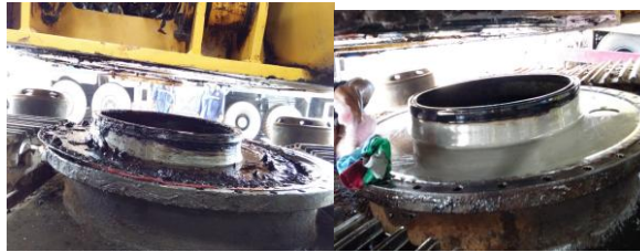
Gambar 13 Disassemble Swing Circle Tahap 7
