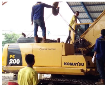
Gambar 11 Disassemble Swing Circle Tahap 5
