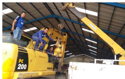
Gambar 9. Disassemble Swing Circle Tahap 3
