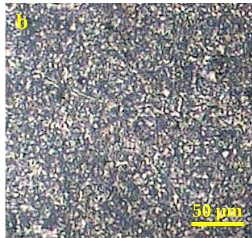
Gambar 13. Struktur Mikro daerah HAZ (a.) Raw material (b.) Normalizing (c.) Annealing
