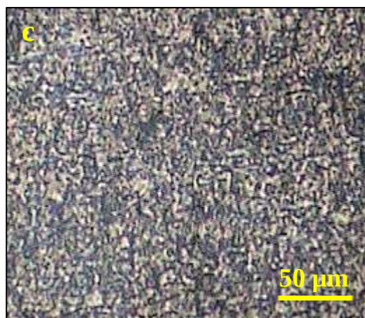
Gambar 14. Struktur Mikro daerah Las (a.) Raw material (b.) Normalizing (c.) Annealing
