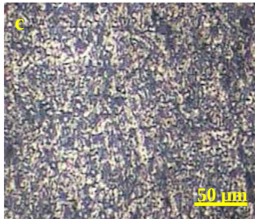
Gambar 13. Struktur Mikro daerah HAZ (a.) Raw material (b.) Normalizing (c.) Annealing
