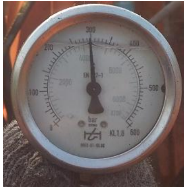
Gambar 12 Tekanan oil hydraulic 300 bar.
