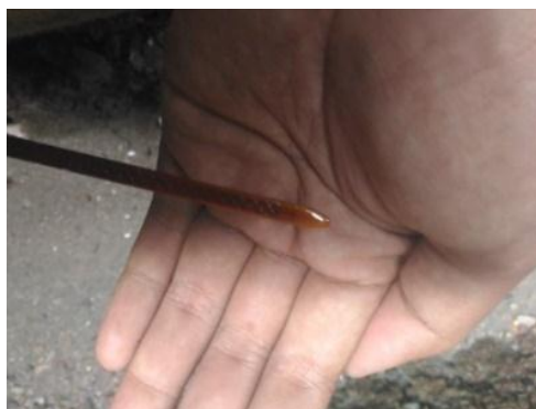
Gambar 19 Volume oil gear swing reduction berkurang.
