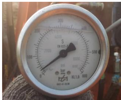
Gambar 11 Tekanan oil hydraulic 20 bar.
