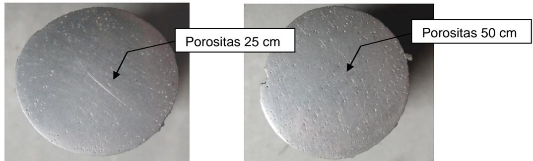
Gambar 9 Porositas specimen
