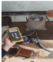
Gambar 10. Mengukur temperatur tuang
