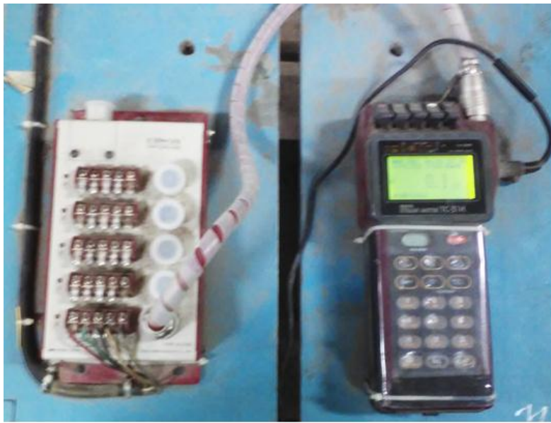
Figure A.5. Digital device for reading the load
