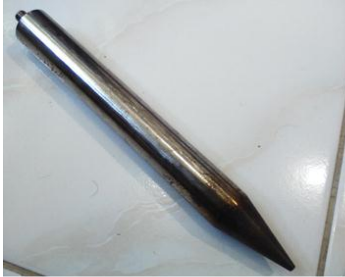
Figure A.3. Piston, attached below the Hydraulic loading machine
