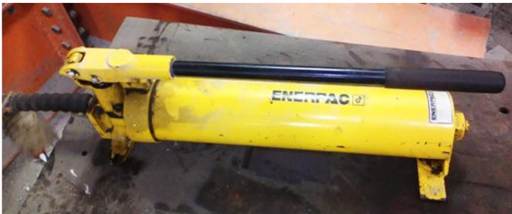
Figure A.6. Hydraulic pump, for giving the load to Hydraulic Loading Machine
