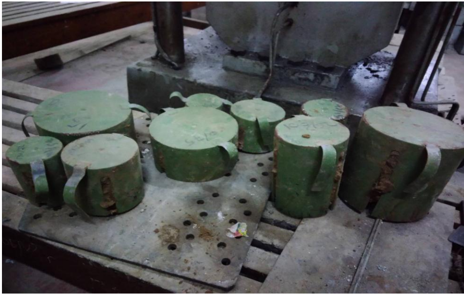
Figure A.1. Partial Skirted footing models
