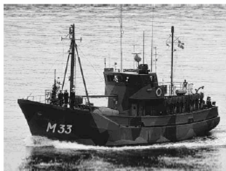
Gambar 1.1. HMS "Viksten" struktur dari glass fiber PVC foam core sandwich .(Bull, 1970)
