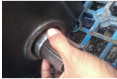
Gambar. 8 proses melepas spacing sleeve dan copper shaft bush
