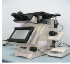
Gambar 6. Inverted metallurgical microscope (Lab.Teknik UGM. Yogyakarta., 2011)
