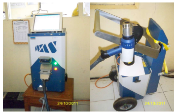
Gambar 5. Optical emission spectrometer (Lab. Pol. Man. Ceper, Klaten.,2011)
