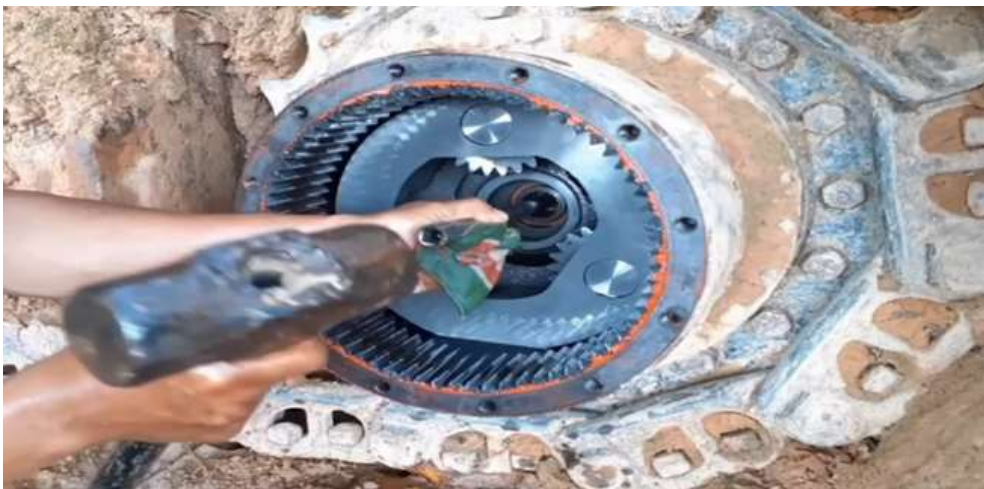
Gambar 9. Proses Pelepasan Drive Shaft
