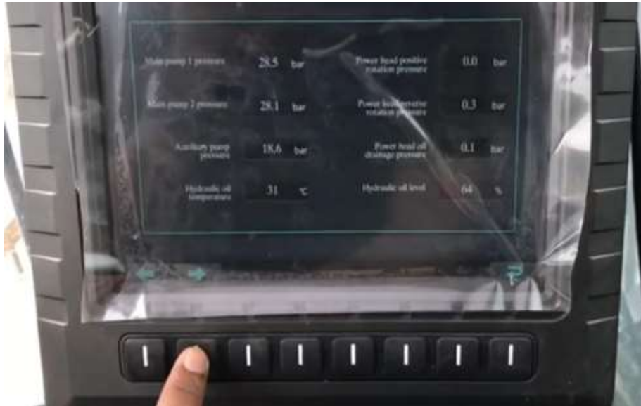
Gambar 2. Tekanan oil hydraulic
