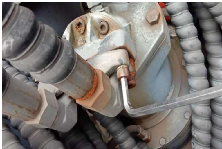
Gambar 5. Melepas hose assembly
