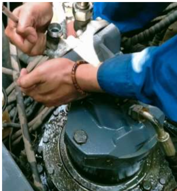
Gambar 11. Memasang hose assembly
