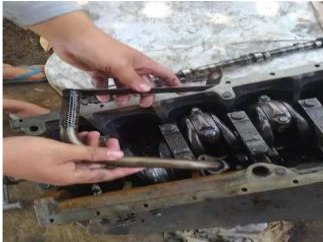
Gambar 3. Proses assembly inlet pipe
