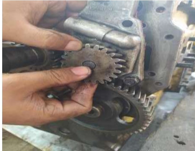
Gambar 1. Proses assembly oil pump ke engine
