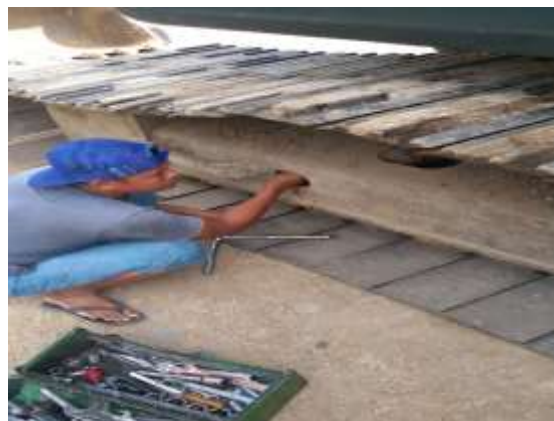
Gambar 7. Melepas grease valve
