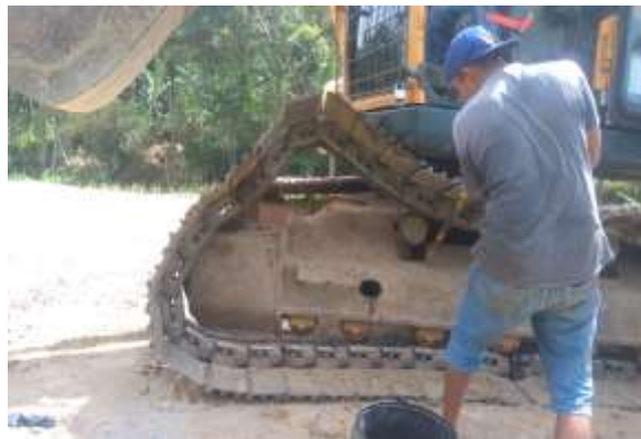
Gambar 9. Proses pelepasan track shoe assembly
