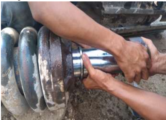
Gambar 19. proses pemasangan rod kedalam cylinder recoil spring
