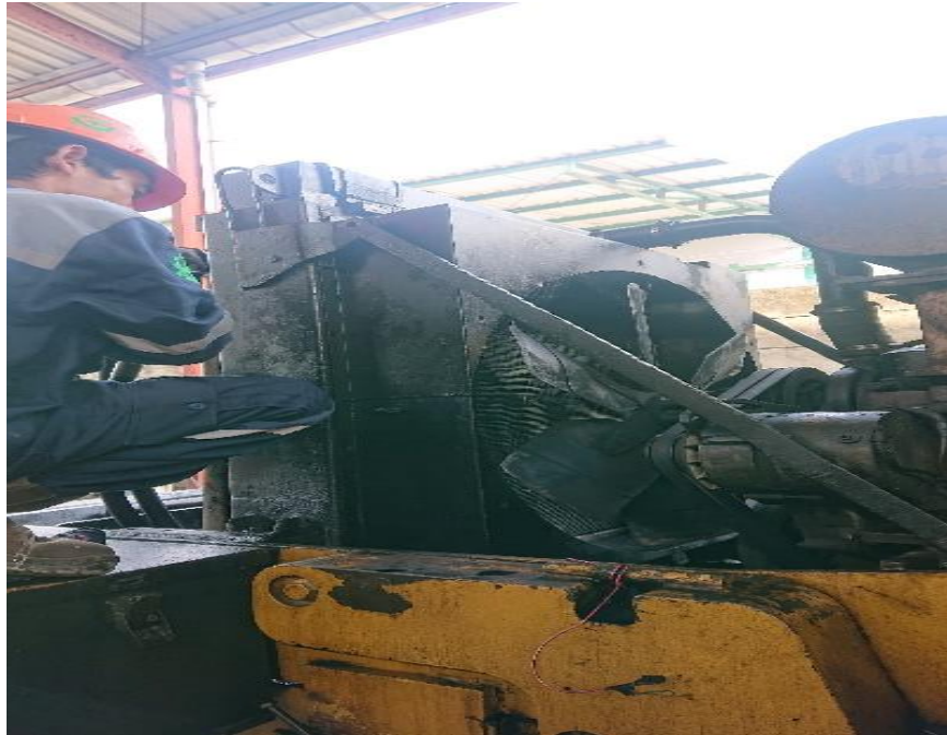
Gambar 4.13 Memasang Penahan Radiator
