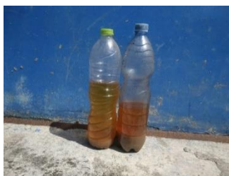
Figure 8. Oil resulting from pyrolysis by burning gasification of sawdust mixed with used oil briquettes
