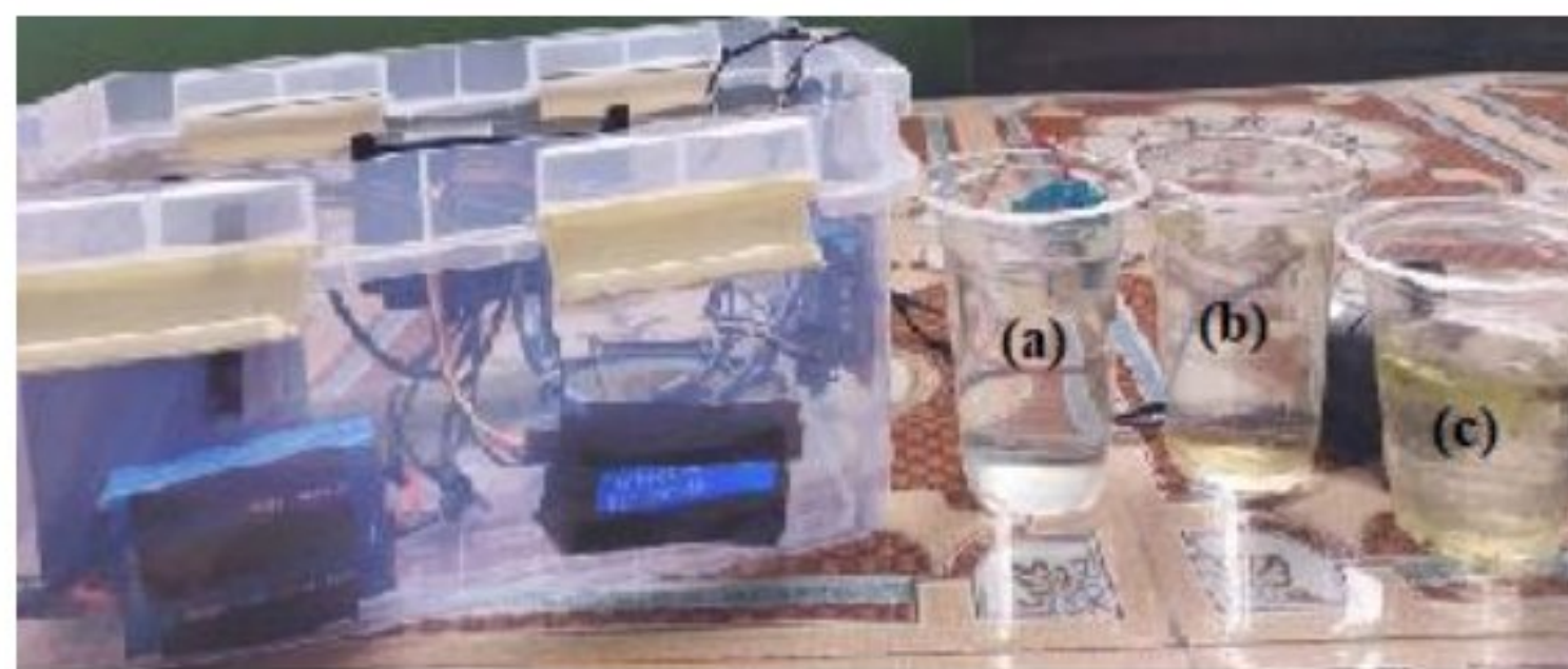
Gambar 10. Pengujian sensor turbidity
