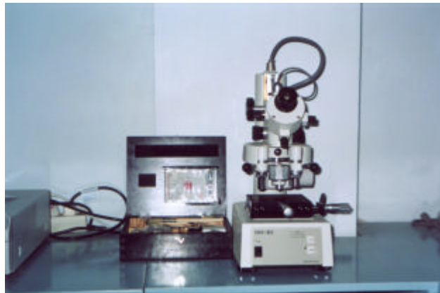
Gambar 3.19. Vickers Macrohardness Tester (Lab. D3 UGM, 2010)
