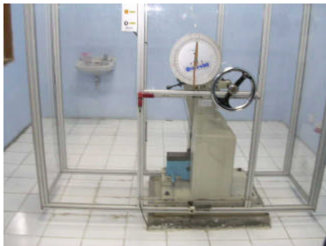
Gambar 3.20. Alat uji impak / Impact Charpy Machine (Lab. D3 UGM, 2010)
