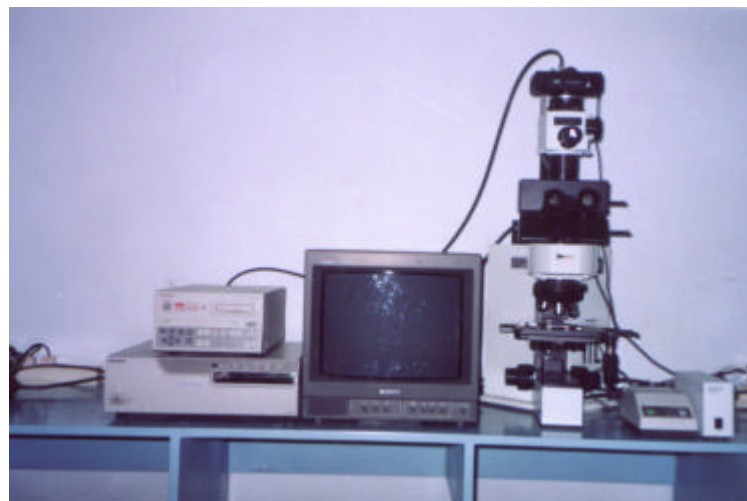
Gambar 3.17. Olympus Metallurgical Microscope dan Olympus Photomicrographic System (Lab. D3 UGM, 2010)
